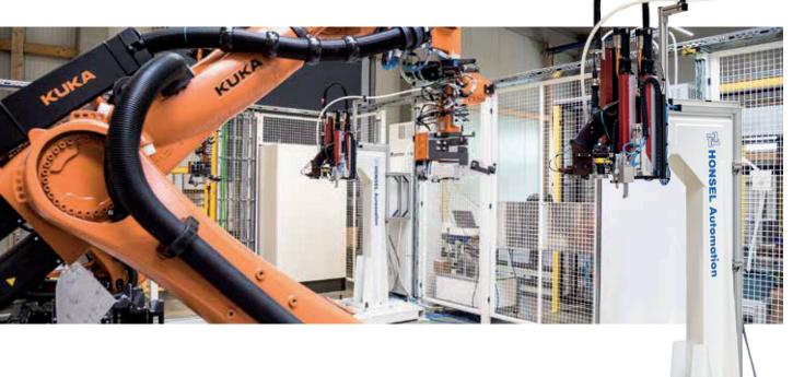
Examples of an automated assembly line for separation, feeding and setting of **HONSEL** coils and **HONSEL** blind rivet studs
